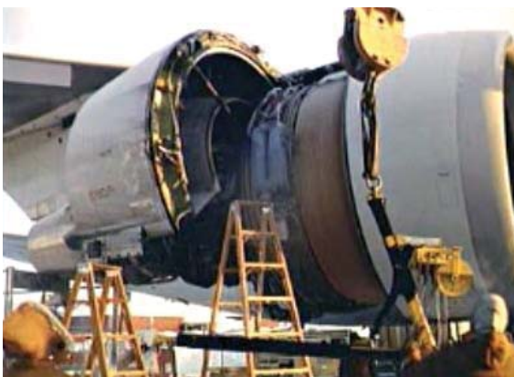
This KLM passenger jet engine has been damaged by volcanic ash.
